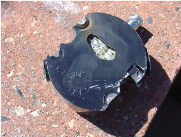
Hole in the resin allowing water ingress
