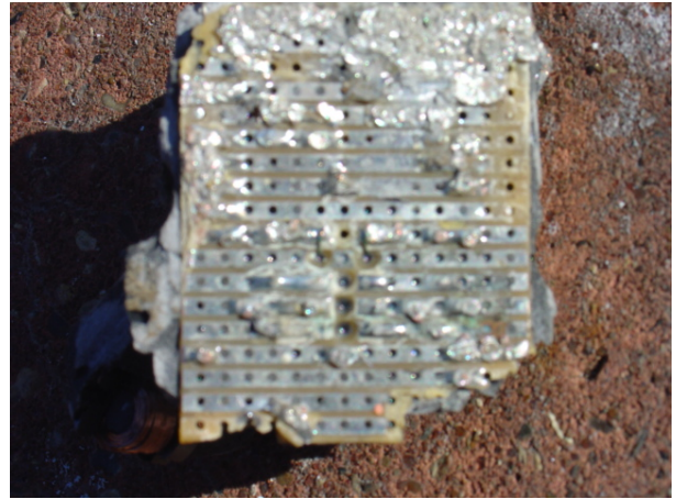
Corrosion on the PCB from water ingress
